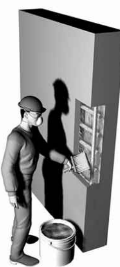
Fig. 6—Treatment of exposed reinforcement.
